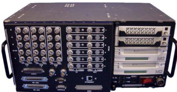
FS-4008 removed from flight case with custom I/O panel & peripherals installed
